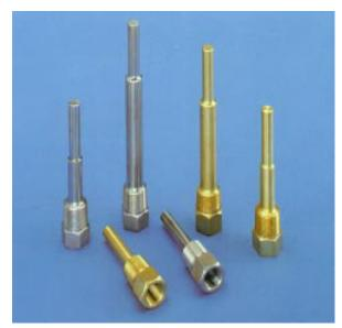
The A-500 Thermowell is machined from a single piece of brass or stainless steel to provide a rugged and leak proof well for MAMAC temperature sensors. Each A-500 Thermowell is precisely machined to 0.255" bore to provide a tight fit for our standard 1/4" O.D. probe. This feature also significantly enhances the thermal transfer from the media to the temperature sensor.
