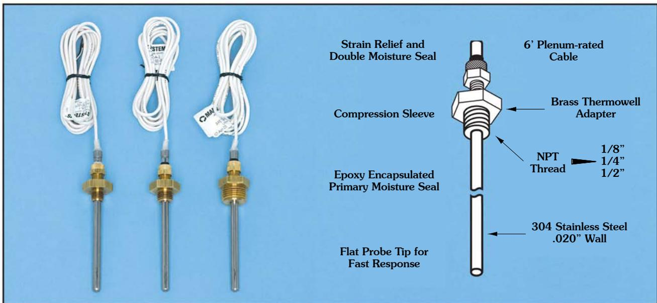
TE-703A Temperature Sensors incorporate unique design features to address the above requirements. Simply screw the brass adapter into the thermowell, insert the probe until it touches the bottom, tighten the compression sleeve, and you are done! To remove the probe for testing, loosen the compression sleeve and just pull it out.
